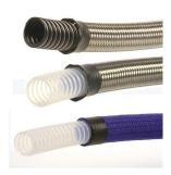
PTFE hoses do not only have an excellent chemical resistance, but are also smell- and tasteless what makes them FDA approved. Because of a low frictioncoefficient, media will not attach to the hose wall.
